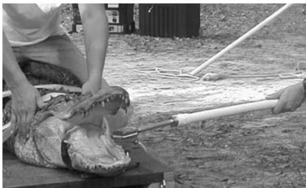
Fig. 3. Bite-force trial on a wild-captured Alligator mississippiensis . The bite plates from the larger of the two transducers are about to be placed unilaterally between the jaws of this specimen. The placement of the device will be centred about the left, 11th maxillary tooth. Note the leather padding on the faces of the bite plates that protect the animal's teeth from damage during trials.
